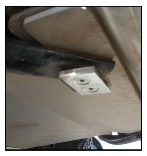
Step ten: Get all of the plates you have mounted so far squared up, and start tightening your bolts from front to rear. Don't forget to tighten the cat tube bars, and remember to anti seize everything.
