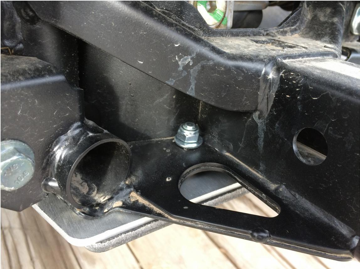
Step thirteen: Now you can mount your top plate. (775T) The front mounting points on the frame are not threaded from the factory. We supply a M6 self tapping bolt for these two mounts. It's easiest to get the threads started before mounting the plate. After getting the threads started put your plate into position and start the two front mounts with the self tapping bolts and cup washers. Leave these loose for now.
