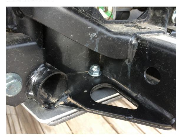
Step thirteen: Now you can mount your top plate. (775T) The front mounting points on the frame are not threaded from the factory. We supply a M6 self tapping bolt for these two mounts. It's easiest to get the threads started before mounting the plate. After getting the threads started put your plate into position and start the two front mounts with the self tapping bolts and cup washers. Leave these loose for now.
