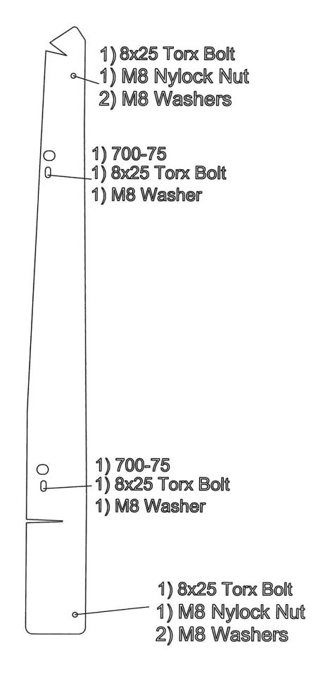
Mount the 700-75 brackets to the side of your machine reusing the existing bolts as shown in the picture below. Be aware there are lefts and rights so make sure it is oriented as shown in the photo.
