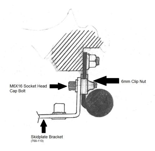
Align the bracket so it runs parallel to the frame tubes. It is much easier to mount the bracket if the exhaust pipe is removed
