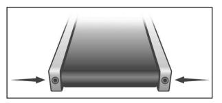
DO NOT OVER TIGHTEN – Over tightening will cause belt damage and premature bearing failure. If you tighten the belt a lot and it still slips, the problem could actually be the drive belt—located under the motor cover—that connects the motor to the front roller. If that belt is loose it feels similar to the walking belt being loose. Tightening the motor belt should be done by a trained service person.
