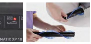
16 Remove brush and check for obstructions, remove if necessary.
