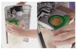
Squeeze green side clips to pull the FA1693 vacuum bag out from the hinges.
