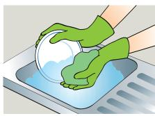
3 Immerse items for 5 minutes. Agitate/wipe as required to remove soiling.
