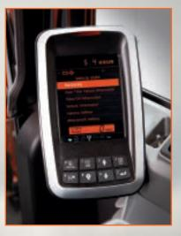
**LCD Self-Diagnostics** An LCD monitor helps you track critical systems in real time and access historical machine alerts from within the cabin.
