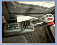
**Fingertip Controls** Auxiliary hydraulic controls are fingertip controlled to deliver precise positioning and easy operation. Variable flow and detent provide more functionality for using different attachments.
