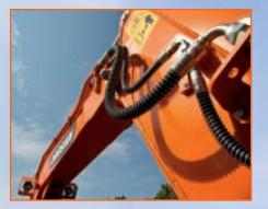
Auxiliary Hydraulic Lines Auxiliary hydraulics are configured with flush face couplers to make quick, easy hose connections when using hydraulic attachments.
