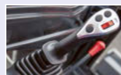
Proportional joystick with auxiliary thumb control
