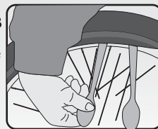
FIGURE B Lift bead with spoons or tire tools.
