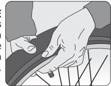
FIGURE E Use thumb to press valve stem through hole in rim. Make certain valve stem is straight.
