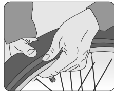
FIGURE E Use thumb to press valve stem through hole in rim. Make certain valve stem is straight.
