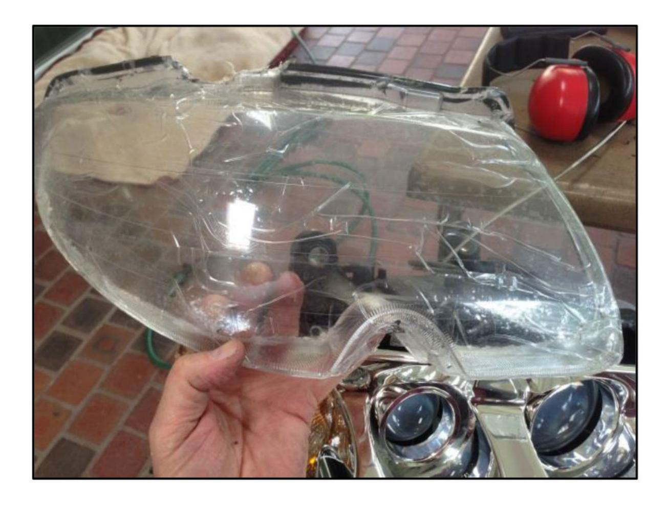
To prevent scratching, cover the headlight lenses with tape and cut off lens with a Dremel or similar high speed tool, keeping as much of the clear plastic intact as possible.
