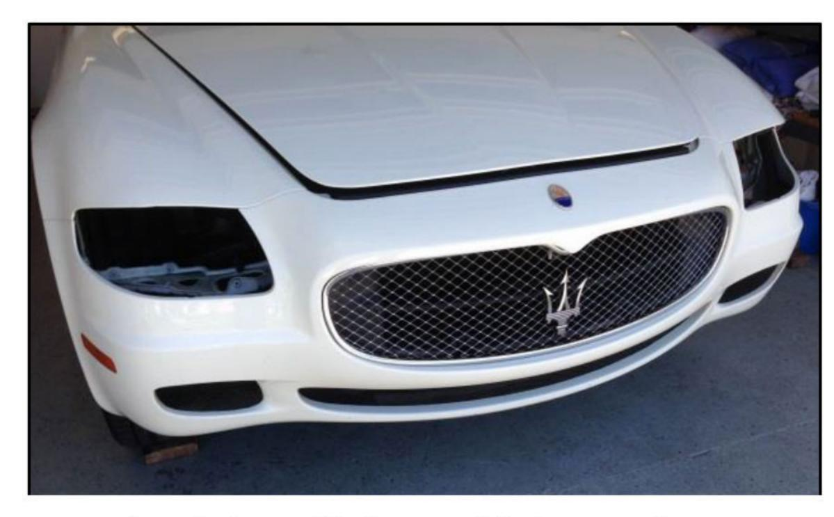
Remove both headlights, which requires access through the wheelwells. Remove the front tires and fender liners. Remove engine covers and release headlight adjusters from inside the engine compartment. Disconnect headlight washer reservoir fitting and all electrical connectors.
