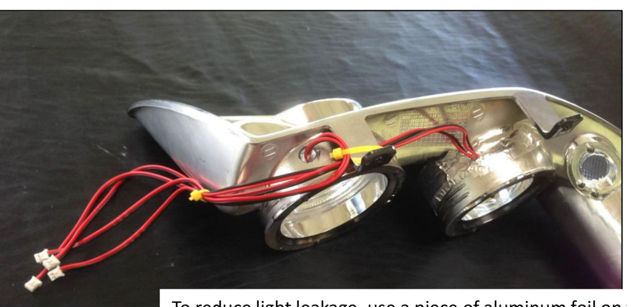
To reduce light leakage, use a piece of aluminum foil on the low beam cutout area after the LED ring is installed; the foil also fills in the area that can be seen from the outside of the headlight housing after reassembly.
