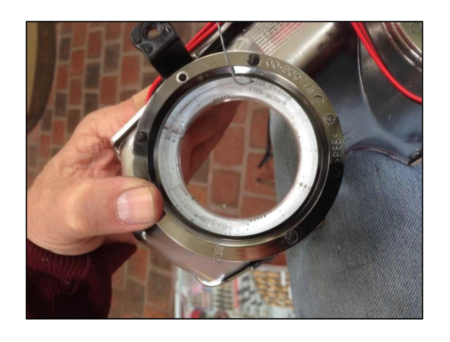
The LED rings that come in the kit are the same size. The low beam opening is very large and the rings will fit over them with ease. Drill a ¼" hole at the top of the housing to run the power wire and glue the rings in place, using the back of the opening to make sure the ring is centered, as shown.
