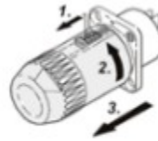
discharge the power cable
