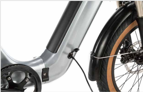
A. Recharge the battery on e-bike directly.
