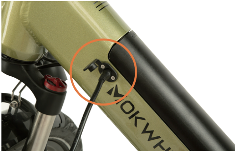
A. Recharge the battery on e-bike directly.
