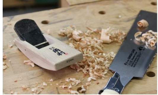
The arc-shaped body of plane
