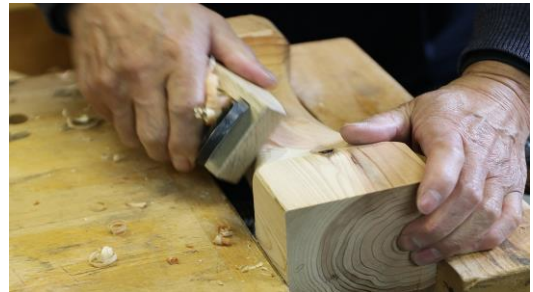
It can finish wood to a curved surface
