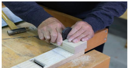
This plane is used to adjust the bottom surface of the plane base.
