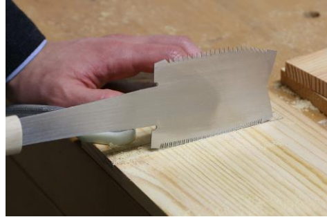
For cut holes, mortises, grooves in mid-panel
