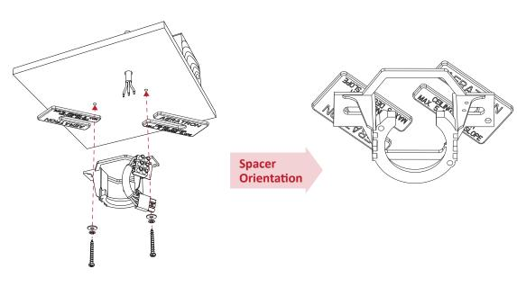
Insert the two Ceiling Spacers between the Hanger Bracket and the Ceiling, in the orientation as shown above to support the frame of the Hanger Bracket.
