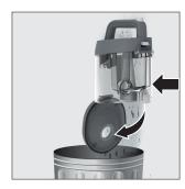
**STEP 4:** Press the dust bin lid button to release the bin lid.
