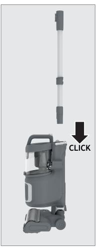
STEP 3: Fit the handle assembly into the wand.
