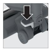
STEP 3: Remove the main unit from the nozzle.
