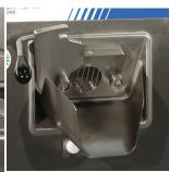
**PRATICA, TELME** batch freezers with vertical cylinder: gelato is effectively mixed during the preparation. The beater pushes the product upwards then gravity brings it down again.
