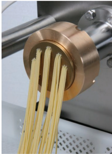
Extrusion of long pasta
