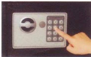
2. Enter the desired code (3-8 numbers) and confirm using "E" button
