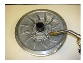
1. Remove driven clutch. Set driven clutch on a workbench with the backside facing up. Using a black marker pen, make a mark on the stationary and movable sheaves so that when you are assembling the clutches that they stay in balance. Next disassemble driven clutch by heating the 4 screws, one at a time with a butane or map gas torch for about 20 to 25 seconds each to
