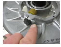
cloth and acetone or brake cleaner, remove all dirt and belt deposits on clutch sheaves. Inspect the moveable sheave bushing for wear and replace it if it is worn.
