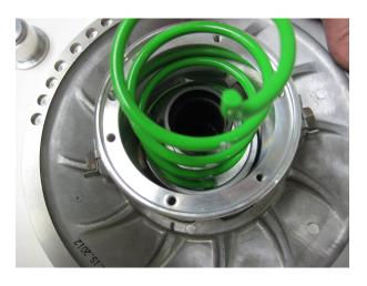
foot lbs. of torque). Note: Make sure that you align the balance marks made in step #1 to insure the clocking of the movable and stationary sheaves are assembled correctly to keep the clutch in balance.
