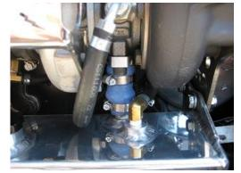
bolt. Over tightening of the three (3) bolts will cause the rubber to smash out and will negate the anti-vibration feature of the rubber grommets. Next
