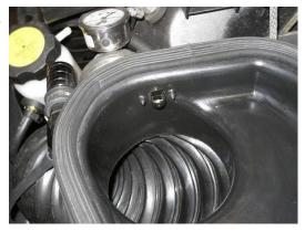
1/2 inch drill bit and drill a hole in the bottom of the 4" X 3" rubber elbow to allow water to drain out. The hole is located in the rubber hose at the lowest point in the hose, close to the inlet of the turbo charger. If this step is not performed, water could puddle and freeze, turning to ice and damage the compressor wheel of the turbo.
