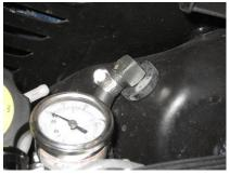
hand and make sure the fuel tank is empty! Then install the rubber bulkhead grommet into the fuel tank and then push the metal bulkhead fitting
