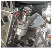
**installation.** Before permanently mounting the oil pump to the foot rest, you will need to connect the oil line hoses to the oil pump. The oil line that is  $5/16 \times 19$  inches long that feeds to the top of the turbo, must be connected to the top of the oil pump outlet (this is the same hose as in instruction #13 above). The bottom brass oil pump barb
