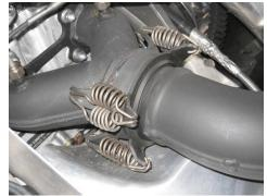
springs in each location to prevent exhaust pipe losing boost pressure. Note if the graph seals are worn; replace them with new seals to prevent boost loss. On 2010 models, the exhaust stinger must be cut off at the factory weld and you will need to fabricate a new stinger to fit exhaust flange at turbo location. A larger exhaust donut and spring tab and washer are included in this kit.
