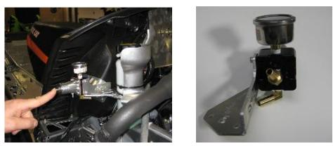
side of the pressure regulator. The center port on the back side is the fuel return back to the top R.H. corner of fuel tank. Then use Teflon tape on the fuel pressure gauge and install it into the top side port of the pressure regulator. Clock the pressure regulator so it positions the hose barb at about the 4 o'clock position, then install the pressure regulator onto the aluminum pressure
