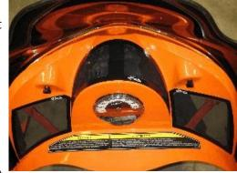
all chips. The holes can now be covered up with a water proof screens that are identical in size
