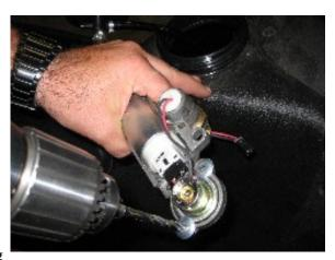
compressed air, blow off the metal chips. Then gently remove the factory pressure regulator by pulling straight out. Account for the two black rubber "O" rings. Using a 1/8 punch; remove the
