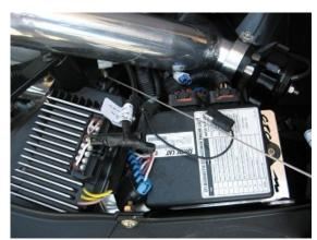
remount the ECU to the forward portion of this bracket. Then reinstall Phillips head screw into the side tab.
