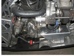
end wrench. The other coolant line, which has a straight end on it must be extended with a 5/16 to 5/16 brass coupler, a 5/16 id X 13 inch hose and Otiker pinch clamps, along with a 90 degree
