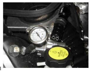
the rope several more times. There has to be at least 20+ lbs of fuel pressure for the engine to start. As soon as the engine starts, you must hurry and re-set the fuel pressure to 36 to 38 psi at a
