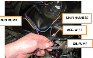
flat" accessory plug outlet located by the chain case by the right hand foot toe-hold. The "two-way flat" connector location provides power from the "lighting coil" and is converted to DC power via the new AC to DC power kit that replaced the factory voltage regulator. This new location will provide enough amps to power the more powerful fuel 6.6 amp CPC high volume fuel pump.
