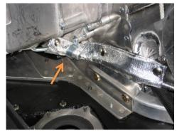
oil injection line. Using a Torex T30 screwdriver, remove the lower R.H. bolt, then attach the band clamp to the bottom bolt of the chain case (see photo). This will prevent the turbo muffler from melting this oil hose. Note: the oil injection hose must be protected and never touch the muffler or the oil injection hose will be damaged and leak oil causing engine failure!
