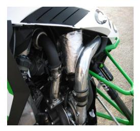
charge tube. Now tighten all bolts securing the compressor housing to the center section of the turbo. Secure all hoses and tubes with CPC provided hose clamps.
