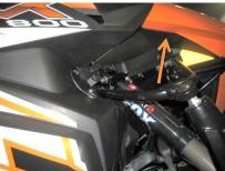
compartment. Clean and inspect drive and driven clutches if you have a lot of use on the snowmobile. Next siphon all the gas out of the fuel tank. Remember that this turbo charged snowmobile will now be using higher octane fuel unless you are using our pump gas actuator at low boost levels. Leave the fuel tank empty as the fuel pump will need to be replaced later in these instructions. Remove both left and right hand side panels.
