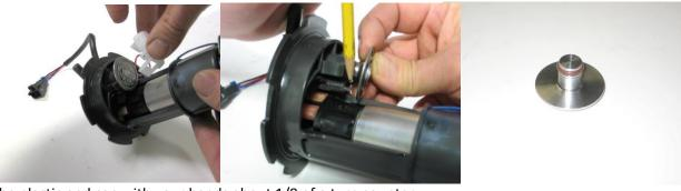
the plastic end cap with your hands about 1/8 of a turn counter clock wise as view from the exit end of the pump. (See photo). Then pull the plastic end cap off and pull the stock pump out of the pump assembly after the electrical terminals are removed. In reverse order, install high volume fuel pump by attaching the electrical wires, then slide the pump into the black rubber hose nipple in the inside of the pump assembly and reinstall the plastic end cap. From the CPC supplied parts, find
