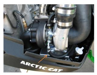
extended with a preassembled 5/16 id X 13 inch long hose that has a brass coupler and 90 female water fitting already attached to it. Using an Otiker pinch clamp, attach the 13 inch long extender hose to the straight factory hose end. Now route the hose in from the front of the engine, then towards the turbo,
