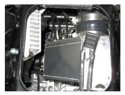
a 5mm Allen wrench. As an assembly, install the throttle bodies and charge box into the rubber intake manifolds and retighten the 2 Philip screws. From the supplied parts, find the rubber snubber attached to a thick cupped aluminum washer and insert the rubber end up through the bottom of the existing 1.375 diameter hole in the front of the bulkhead and attach the rubber snubber to the charger box.
