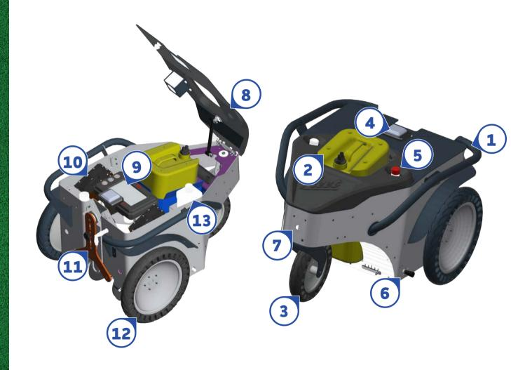
Handles to make transporting your RoboLine easier Carries RFU Jerry cans with a capacity of 10L or 12.5L **Solid Rotating Wheel GPS Antenna Emergency stop button** Easy line width adjustment Ultra sonic sensor protection Easy access to the machine Storage and home for SPIKE Removable batteries 10 Simplistic nozzle maintenance Non Puncture Wheels
