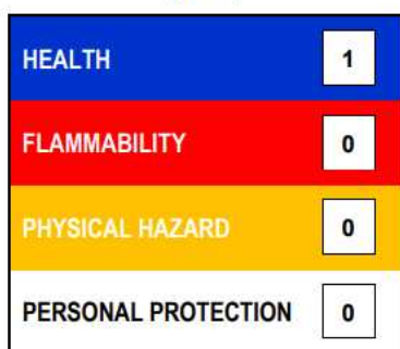
Hazardous Materials Identification System (HMIS)
