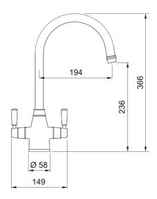
Gloriana Decor Steel tap, quarter turn ceramic disc mixer, Overall height 366mm, twin lever, Ceramic valves, suitable for low pressure systems.
