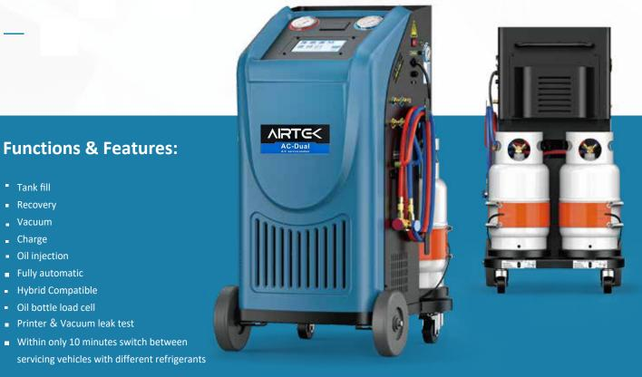
AC-Dual20 is an ideal option for workshops that have requirements of handling both R-134a and HFO-1234yf refrigerants. The loss of refrigerant is minimized to less than 50 gram at shifting from one refrigerant to another, and deep internal evacuation ensures zero cross contamination between the two refrigerants. The machine is equipped with two refrigerant tanks, which saves the operators' time of replacing tanks.
