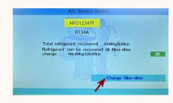
• If touch screen, switch on the machine and select "Change filter-drier". Then 6-digit code will appear on the screen.
