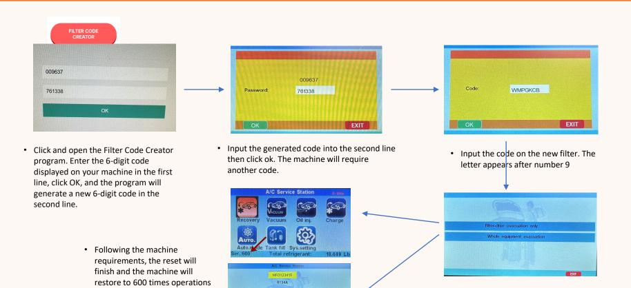
Normally select "Filter-dryer evacuation only". The machine will evacuate one
