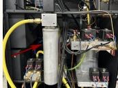
· Open the machine's casing and replace it with the new filter
