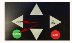
Hold down the left arrow and green Enter button simultaneously, then power on the machine until a 6-digit code appears on the screen
