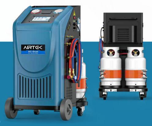
AC-Dual20 is an ideal option for workshops that have requirements of handling both R-134a and HFO-1234yf refrigerants. The loss of refrigerant is minimized to less than 50 gram at shifting from one refrigerant to another, and deep internal evacuation ensures zero cross contamination between the two refrigerants. The machine is equipped with two refrigerant tanks, which saves the operators' time of replacing tanks.
