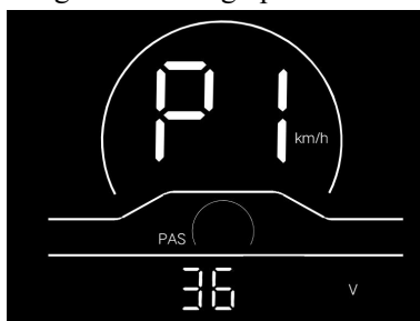
Fig. 4-1 Rated Voltage Setting Interface
