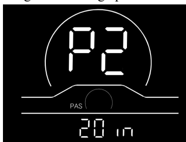
Fig. 4-2 Wheel Diameter Setting Interface
