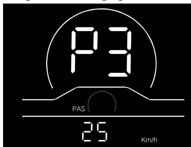
Fig. 4-3 Speed Limit Setting Interface
