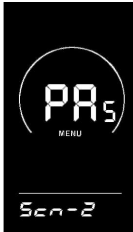
Fig. 8-7 Assistance sensor sensitivity setting interface
