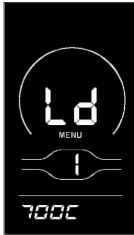
Fig. 7-1 Wheel Diameter Setting Interface
