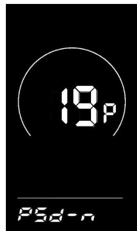
Figure 6-20 Power-on Password Activated interface
