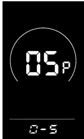
Figure 6-6 PAS level setting interface
