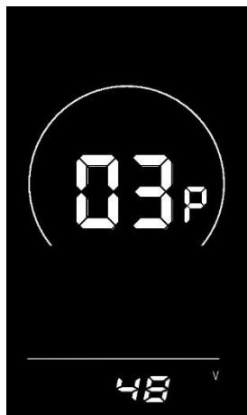
Figure 6-4 Rated voltage setting interface
