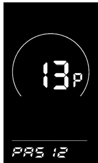
Figure 6-14 Number of pedal assist sensor magnets setting interface
