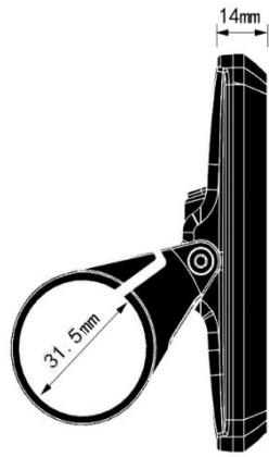
Fig. 3-4 Side View of Display 80C Dimensions
