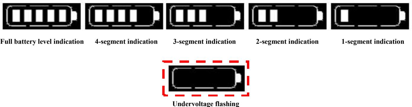
Fig. 5-5 Battery Level Indicator Interface
