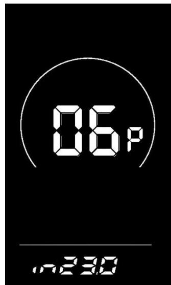
Figure 6-7 Wheel diameter setting interface
