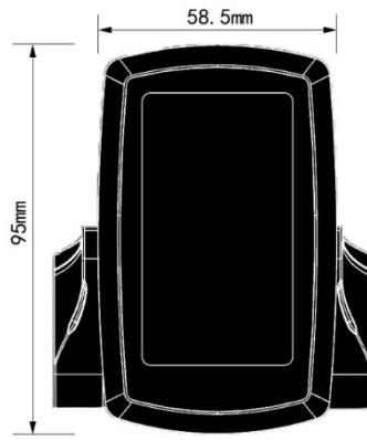
Fig. 3-3 Front View of Display 80C Dimensions
