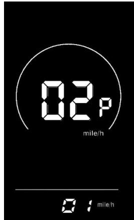
Fig. 6-2 Imperial System Setting Interface
