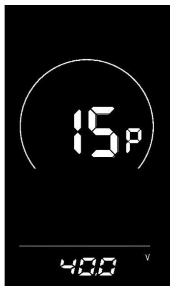
Figure 6-16 Battery under voltage value setting interface
