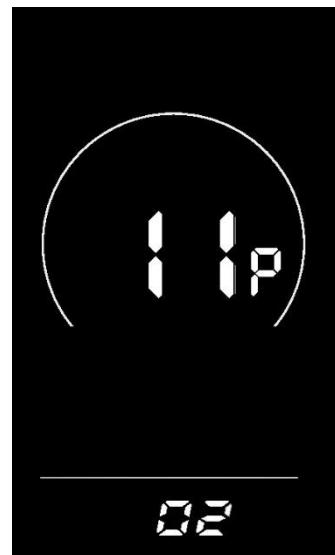
Figure 6-12 Pedal assist sensitivity setting interface
