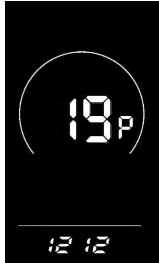
Figure 6-22 Power-on password setting interface
