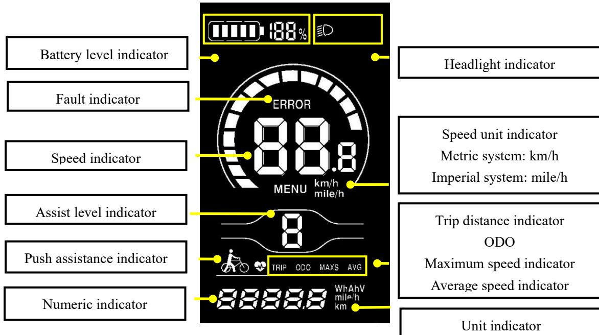
Fig. 4-1 Functional Area Layout Interface of Display YL80C
