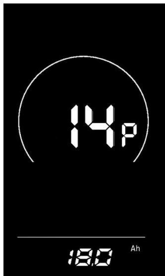
Figure 6-15 Controller current limit setting interface
