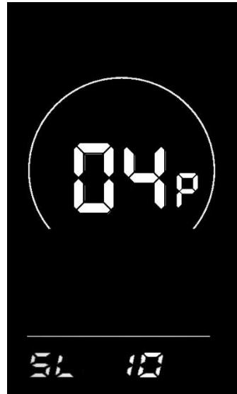
Figure 6-5 Auto Power Off Time Setting Interface
