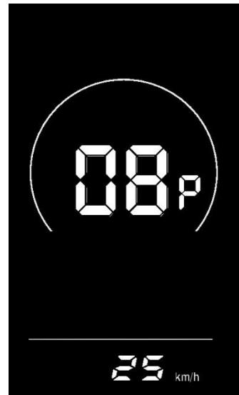
Figure 6-9 Speed limit setting interface
