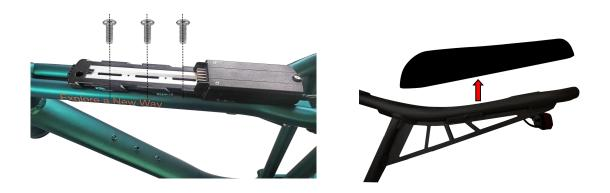
Step 2: Connect the guide slot connecting line to the power equalizer, Battery 1 and battery 2 do not need to distinguish plugs, As shown below;
