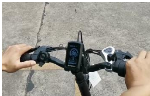
Step3: Turn on the display at the same time, keep holding throttle bar & left brake for 8 seconds.
