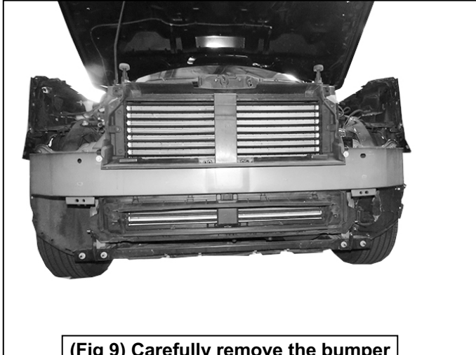
(Fig 9) Carefully remove the bumper and place in a safe location. Remove the (2) outer nuts from the lower crossbar
