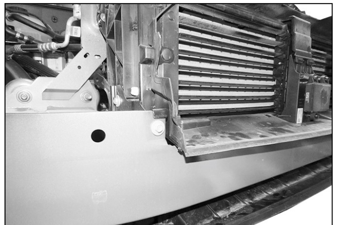
(Fig 14) Locate and remove the bolts in the upper crossbar (Passenger/Right side shown)
