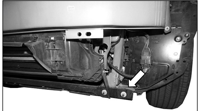
(Fig 10) Temporarily remove the (2) outer nuts from the lower crossbar
