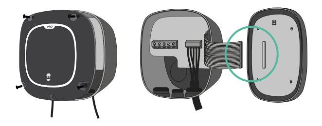
Before proceeding with the installation, power off all the connections.
