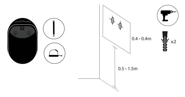
Insert the anchor screws into the fixing holes. Then secure the device to the walls by inserting and tightening the screws.
