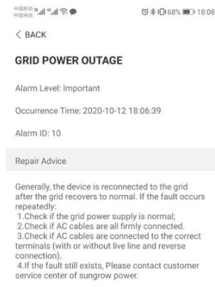
Figure 7-10 Detailed Fault Alarm Information
