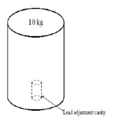
Weight is 190 mm in height with a diameter of 95 mm
