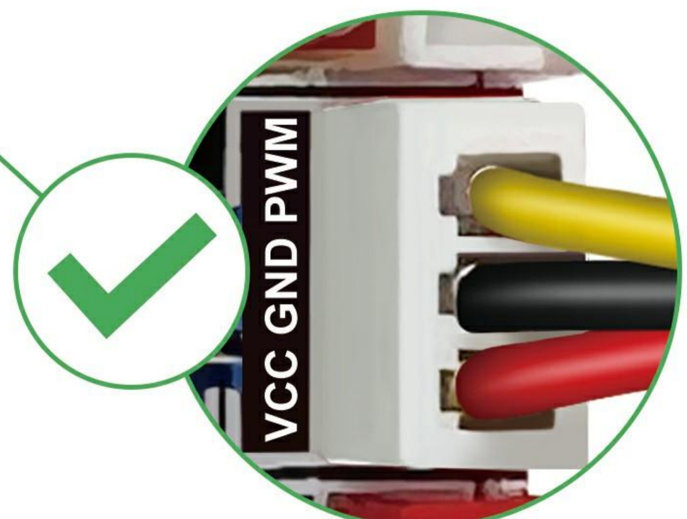
"Red: Power" and "Yellow: PWM" connection correctly
