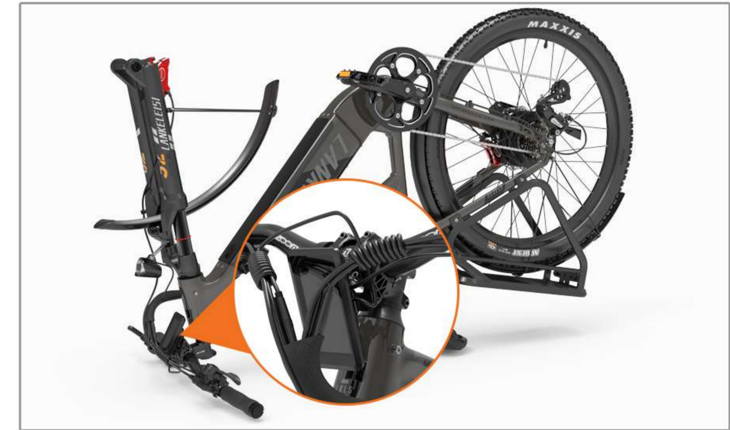
03 Preliminary work for installing front wheel Invert the entire vehicle. Flip the instrument angle to avoid direct contact with the ground
