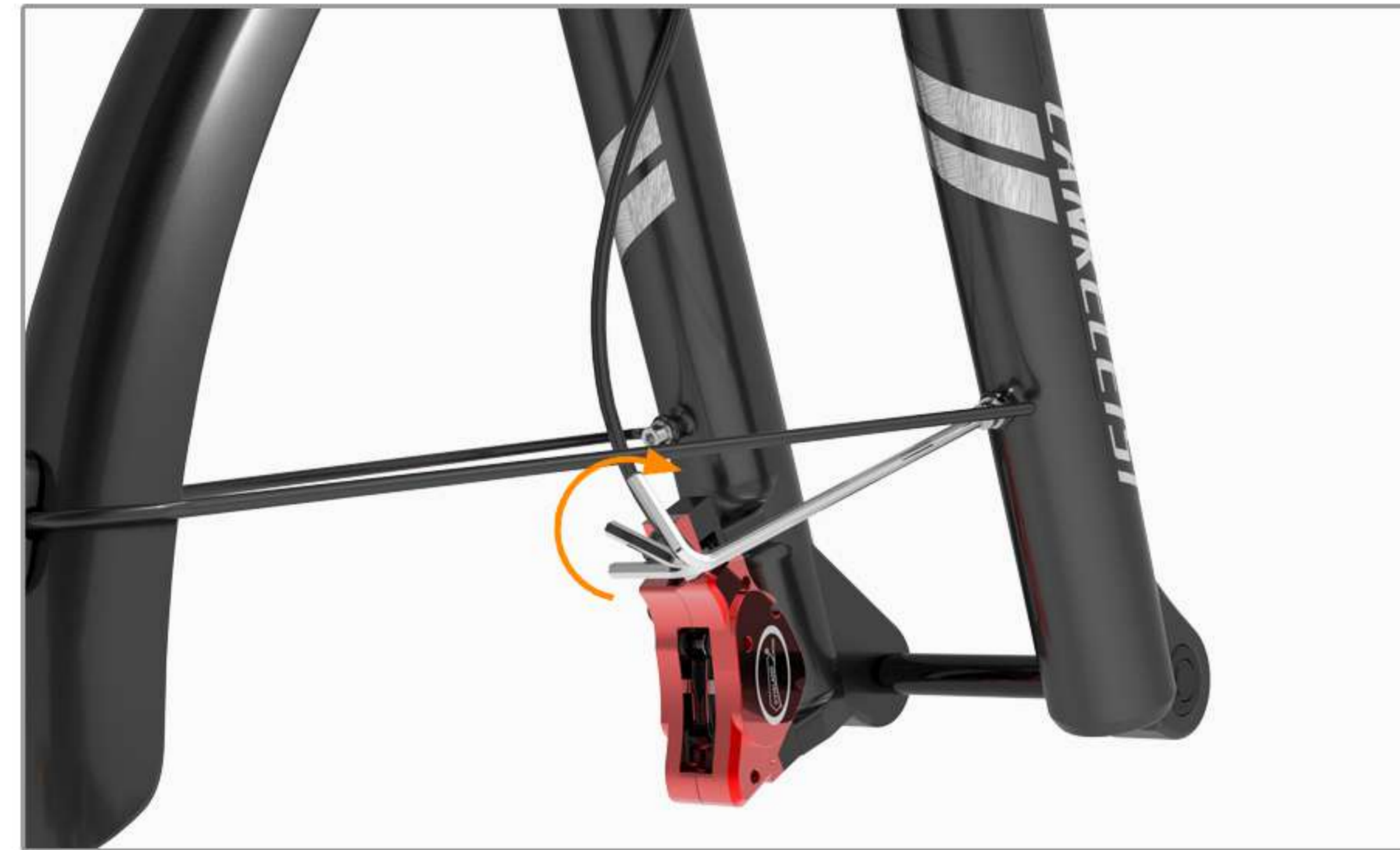
02 Fix the mudguard branches in the correct position and tighten the screws
