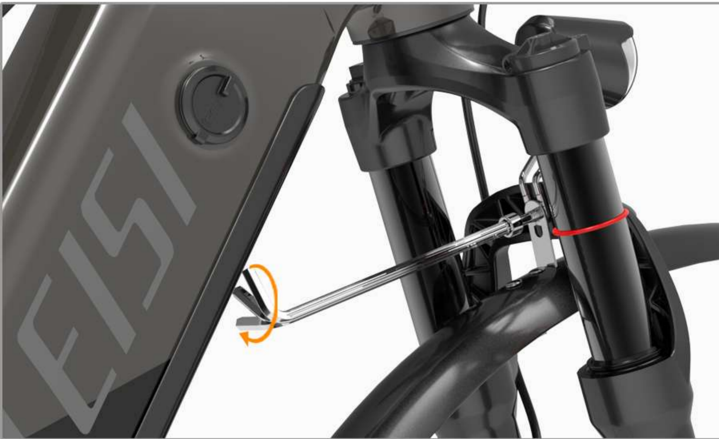
01 Adjust the front fender and headlights to the correct position and tighten the screws
