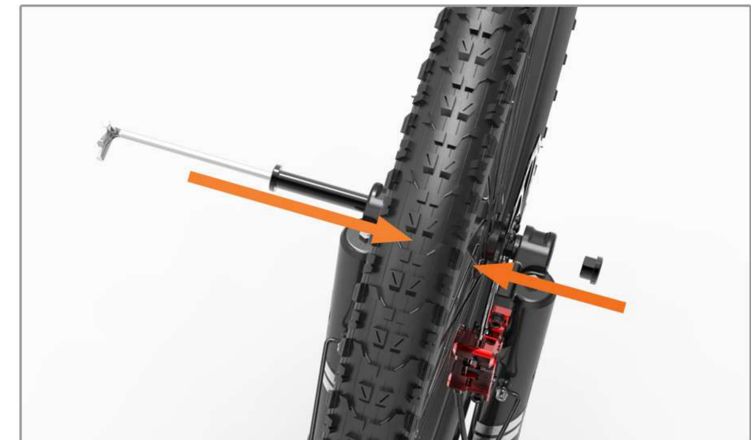
06 insert mounting shaft
