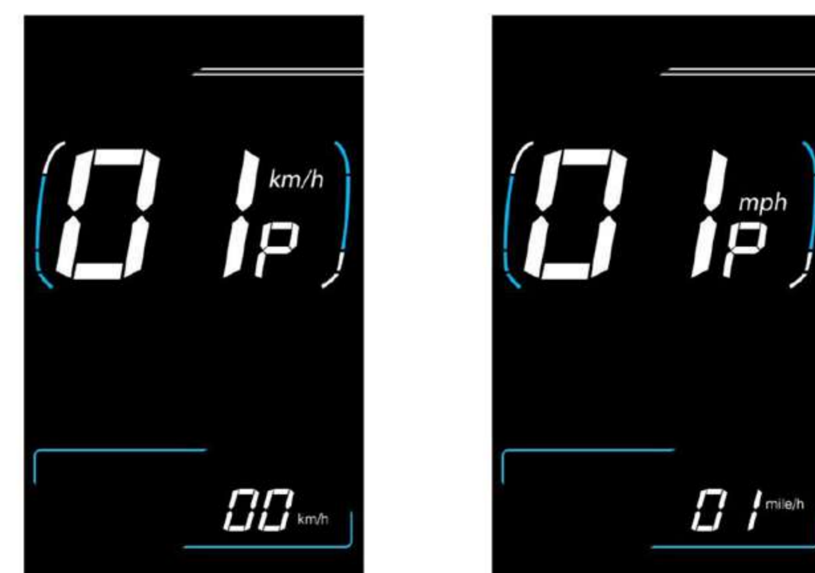
(01P is shown in the picture) Metric and Imperial unit setting interface
