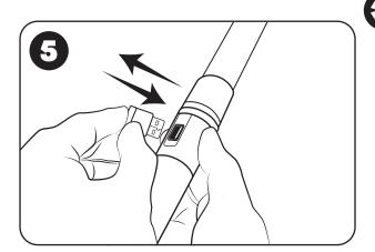
PLEASE READ: Since batteries are brand new, to power up you may need to build a charge. To do this, insert the USB A plug in and out of the battery port very quickly twice, and then you should see your totem power on! Use the remote to change graphics or the SmartApp!
